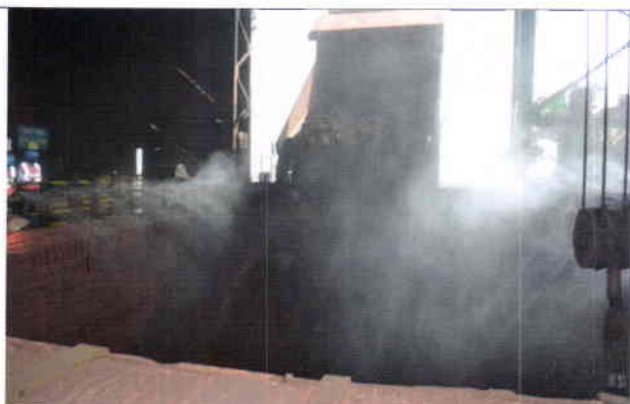
Photograph showing High Pressure Dust suppression installed at Feed Hopper at Hill Top Plant
