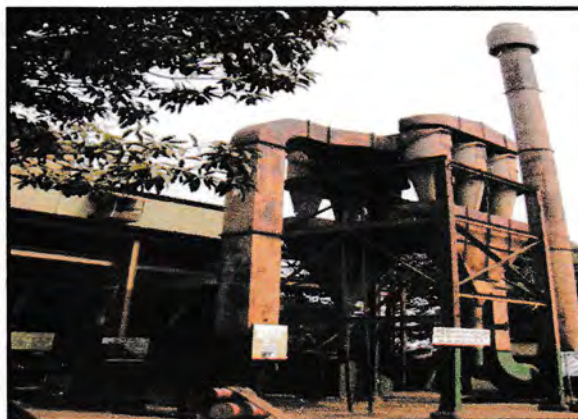
Photograph 6: Dust Extraction System at Crushing Plant
