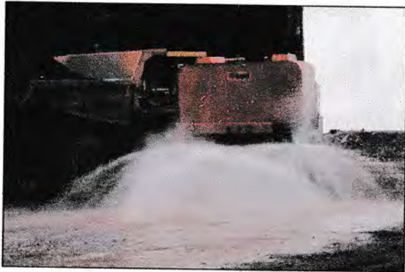
Photograph 1: Haul Road Water Sprinklers
