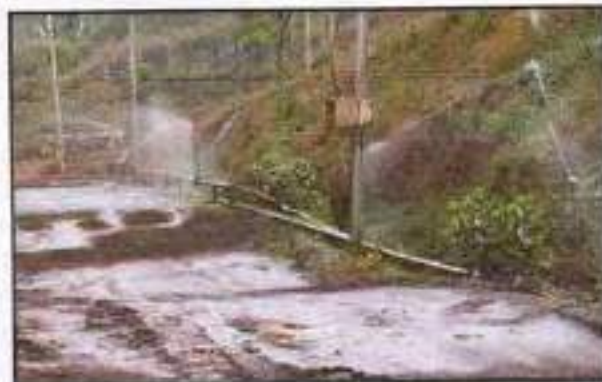
Photograph 2: Permanent Road Sprinklers in Mines
