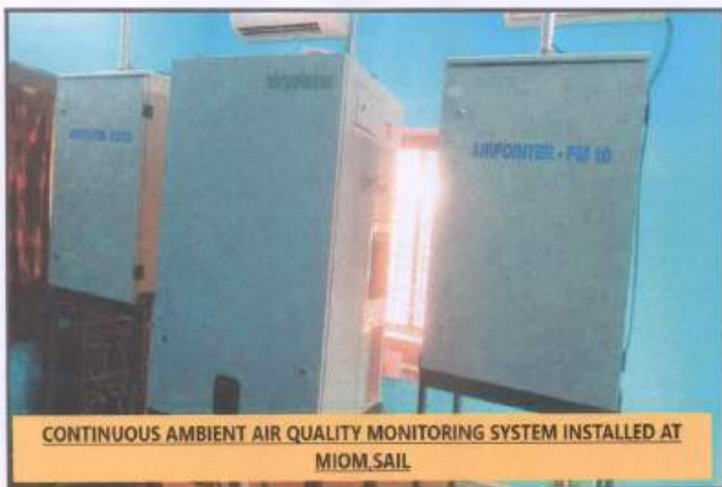
ANNEXURE-21: A- CONTINUOUS AMBIENT AIR QUALITY MONITORING SYSTEM INSTALLED AT MEGHAHATUBURU IRON ORE MINES, SAIL
