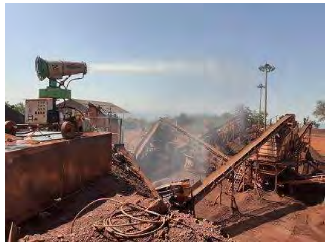
Operation of Mist Cannon at Kalta Block
