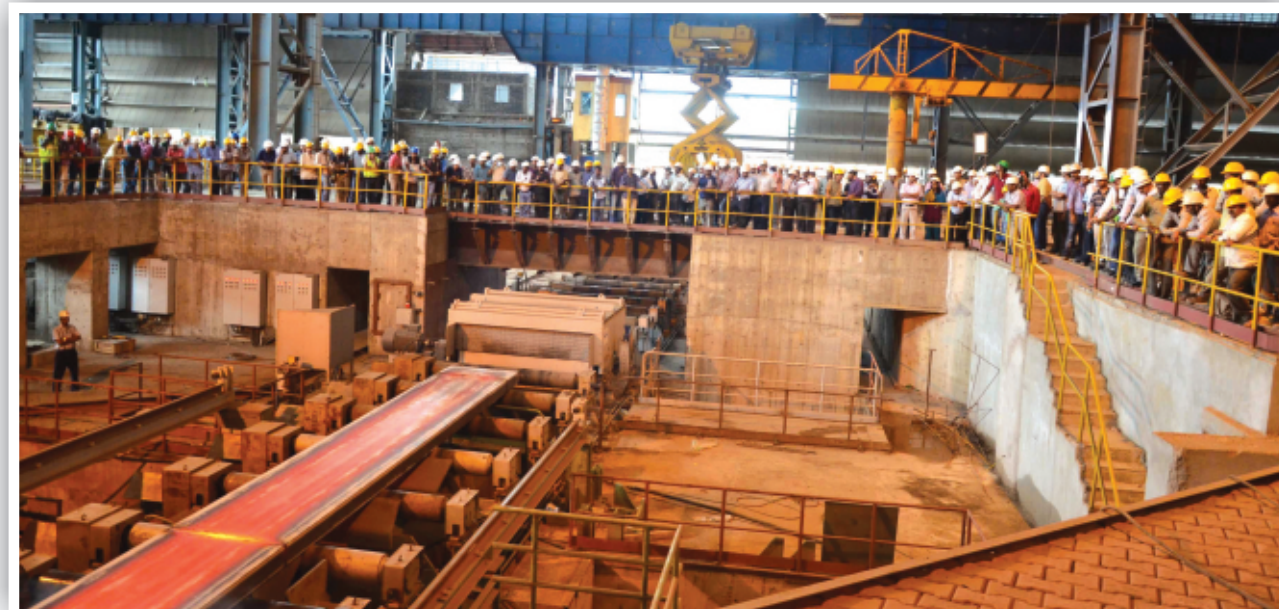
Slabs being produced from the new state-of-the-art slab caster at Rourkela Steel Plant
