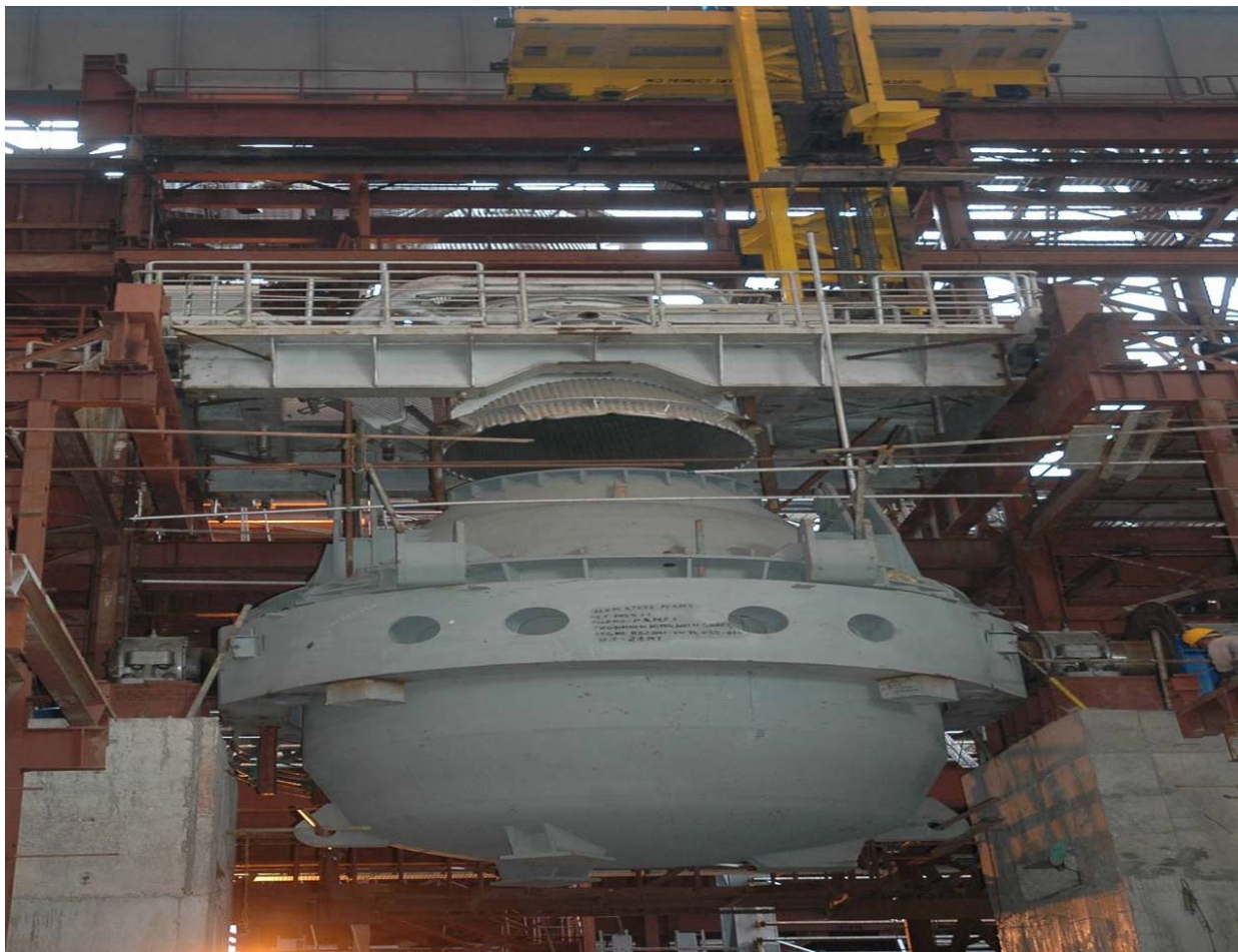
Argon Oxygen Decarburisation (AOD) Refining Converter at SAIL's Salem Steel Plant.
