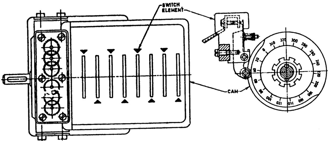
FIG.4 SPINDLE LIMIT SWITCH WITH ROTATING CAM (TYPICAL)
