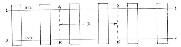
**ON RAIL 1**, point A is high and ON RAIL 2, point B' is high.
