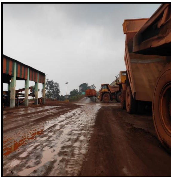
ANNEXURE-8: A- 28 KL WATER SPRINKLER MOUNTED ON DUMPER, SPRINKLING ON HAUL ROAD AT KIOM
