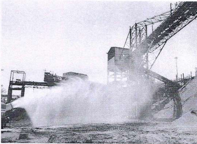
Photograph showing Mist generation for suppression of dust at Ore stockpiles
