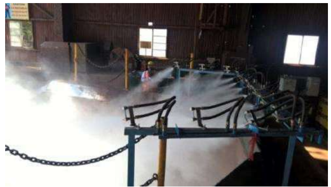
Dry fog Dust Suppression in Crusher, Barsua
