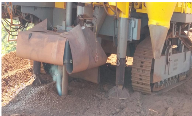
Photograph showing Wet Drilling
