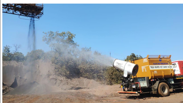
Photograph showing Truck Mounted Mist cannon in operation
