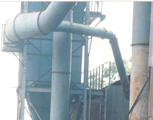
Photograph showing Bag House installed at secondary Crushing Point
