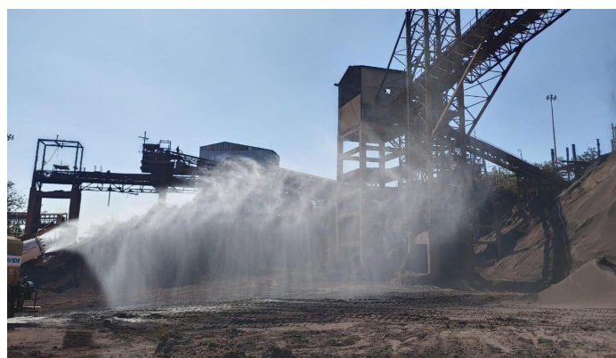
Photograph showing Mist generation for suppression of dust at Ore stockpiles
