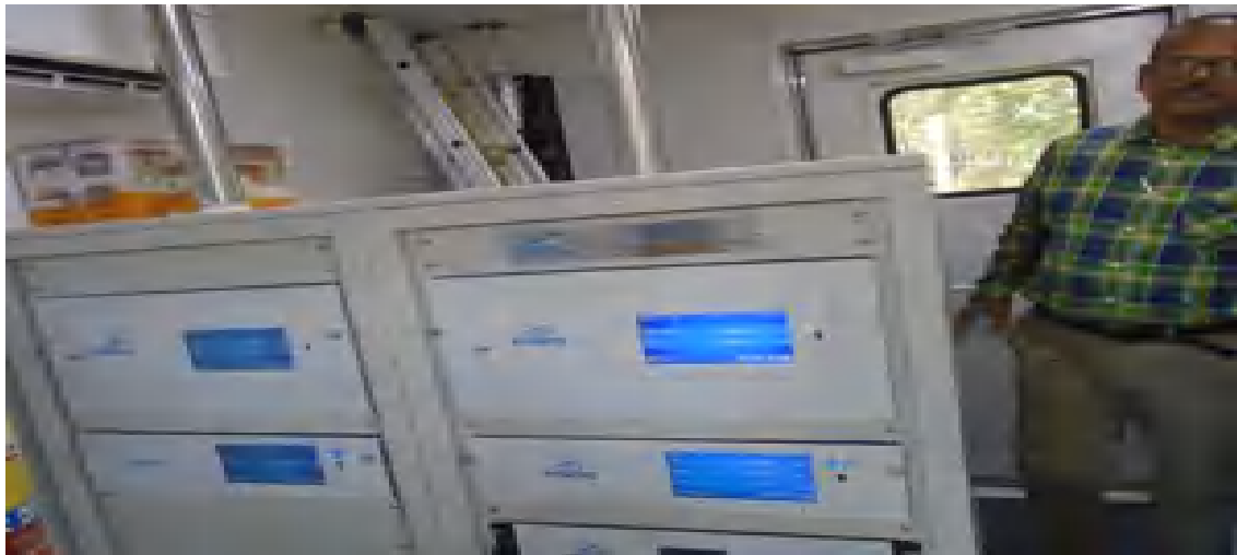
View of online continuous AAQ monitoring station installed at occupational health centre located at Khodgaon.
