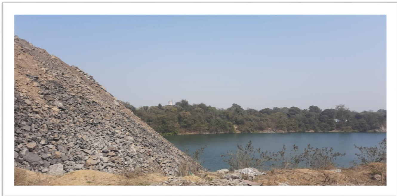
OB was dumped at Old Quarry located within earmarked OB dump Area as per Mining Plan of Tasra.
