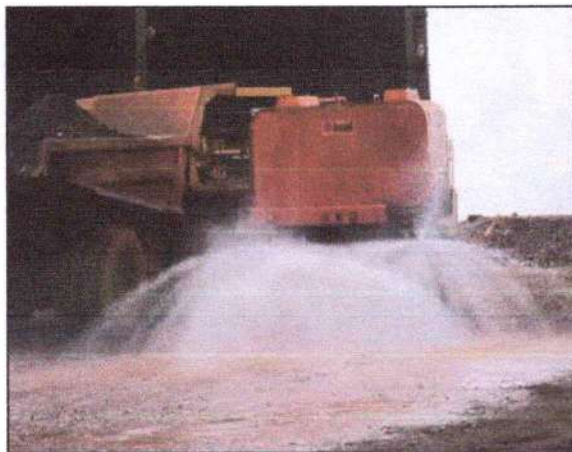
Photos: Water sprinkling through mobile water tanker at mines haul road and near railway siding area.
