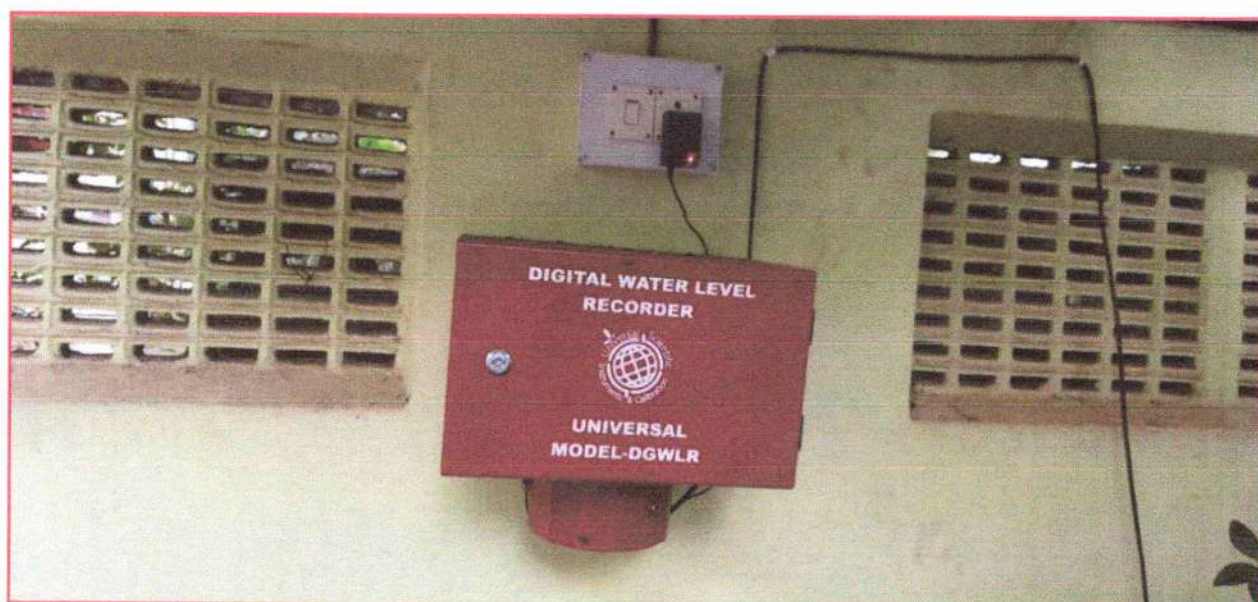
Photo: Real time groundwater monitoring station installed at Director Bungalow and also installed at other two location namely Guasai-Forest Bungalow and DB Annexe
