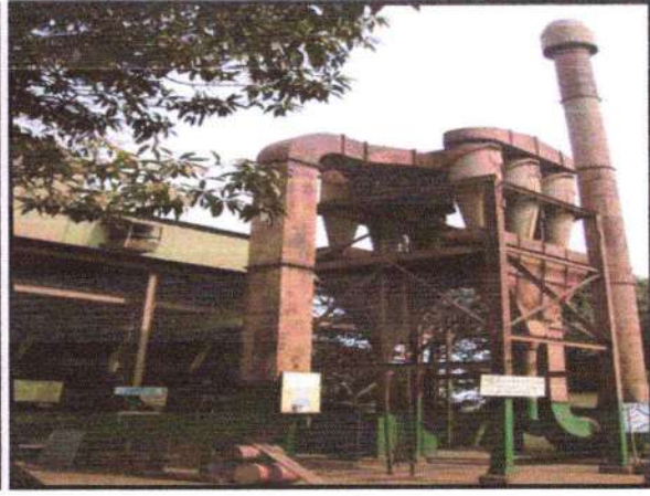
Photo: Dust extraction system at crushing plant.
