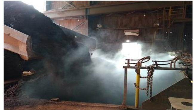
Dry fog Dust Suppression in Crusher, Barsua
