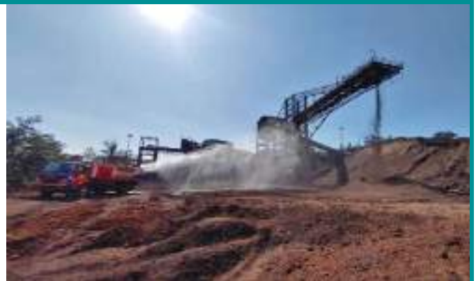
Truck Mounted Mist Canon Deployed at Near Fines Stacker
