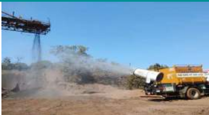
Truck Mounted Mist Canon Deployed at Near Fines Stacker
