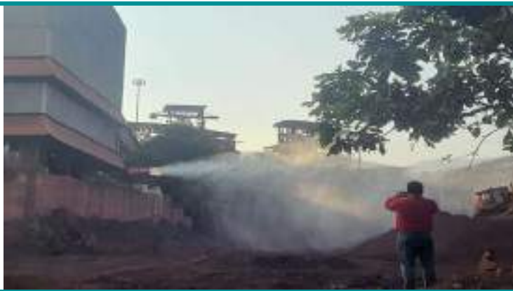
Rotating Fog Canon Installed at Lump Loading Plant
